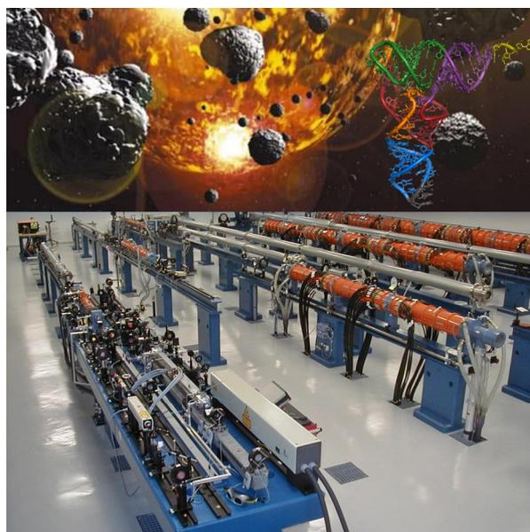
Panel 5. Prague Asterix Laser System (PALS) is a terrawatt iodine laser, which was used to simulate high-energy density processes. The laser shots simulated impacts of extra-terrestrial bodies into the early Earth's atmosphere simulant (Late Heavy Bombardment period). During this process, the formation of organic molecules (as complex as nucleic acid bases) from simple precursors (H<sub>2</sub>O, CO<sub>2</sub>, CH<sub>4</sub>, CO, N<sub>2</sub>) was discovered<sup>38,42–45</sup>
